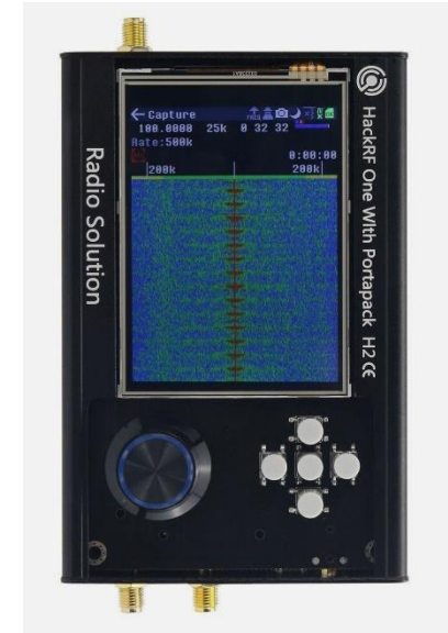
HackRF One Software Defined Radio (SDR)
