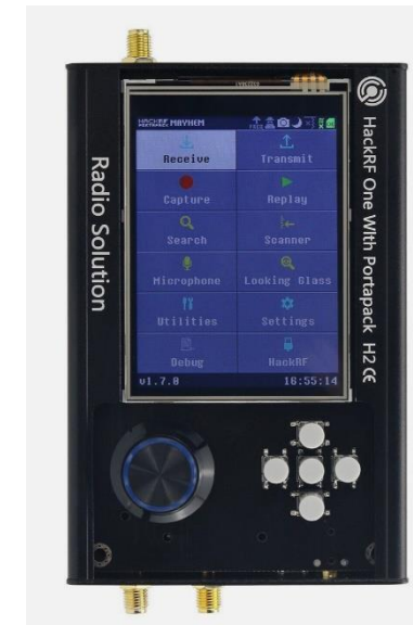
HackRF One Software Defined Radio (SDR)
