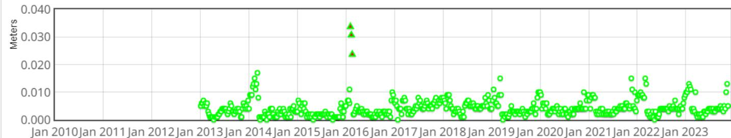
DUBO horizontal time-series in NAD83(CSRS) with velocity model (IFDM) applied
