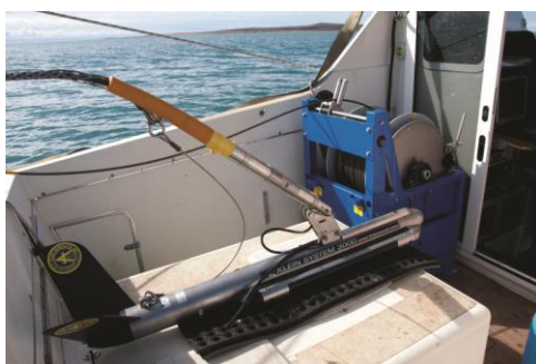
Parks Canada side-scan sonar towfish, cable and winch on the CHS survey launch Kinglett in 2010.
