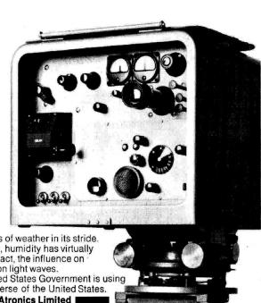
Laser Geodimeter 8 takes all kinds of weather in its stride. And unlike microwave long range measuring, humidity has virtually no effect on the accuracy of a light beam. In fact, the influence on microwaves is about 100 times greater than on light waves.
