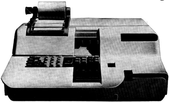
The Programma 101 is not simply an electric calculator. It is a true computer and can solve complex repetitive problems automatically—and almost instantly. It stores, computes, makes logical decisions and prints. Programs are stored on magnetic cards about the size of punched cards. Only vari-
