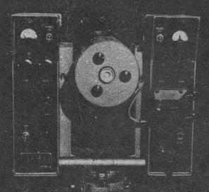
Lightweight 12V rechargable battery pack weighing only 2½ lbs. powers the Model 6.
